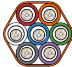
Example - Feeder TWD 14/10mm 7way ABC – 200um 288F ( 7.9mm ID of cable) Total 2,016 Core
