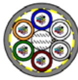
ABC Loose tube 72 core 5.2mm, 21kg/km
